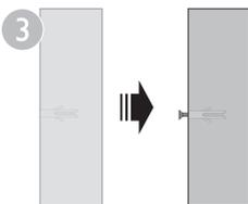
Drill two holes in the wall (7/32" drill bit). If you drill the holes into a stud, insert the screws into the holes.
