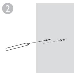
Use a pencil to mark two holes in parallel. Make sure they are the same distance apart as the wall mount at the bottom of the baby unit.
